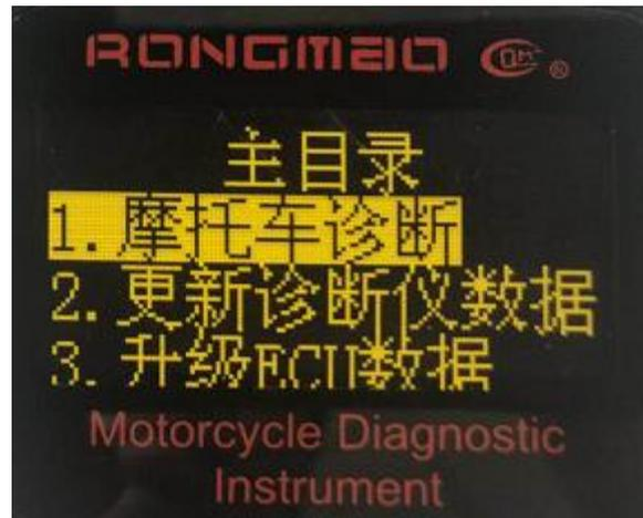
5) Press the [ENTER] key and a diagnostic message can be seen on the display until the vehicle agreement is completed.
